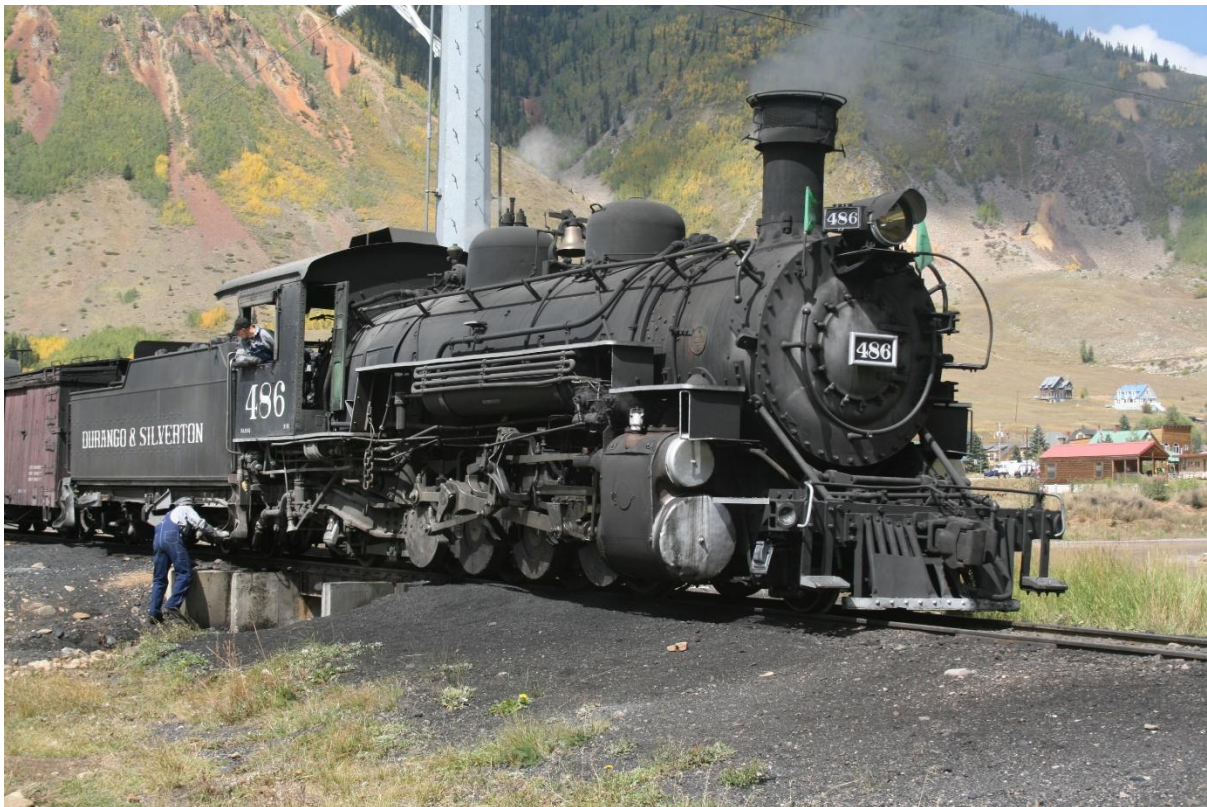
3 ft gauge Denver & Rio Grande class K-36 Mikado #486 (Baldwin, 1925) at Silverton, Durango & Silverton Narrow Gauge Railroad, Colorado, 2009
